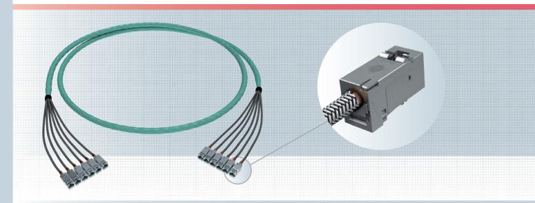
Thanks to its minimal cable diameter and the associated low fire load, the CTCC distribution system is ideal for flexible use in structured building cabling and data centers. Six-fold (6 x 4P) cables leave the factory pre-assembled with fixLink® cable connectors and tested. The maximum length of the multi-cable is 60 meters.
